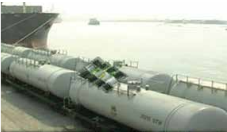
Pressurised fire-proof Wagons in Lagos for conveying oil and gas products across the country
