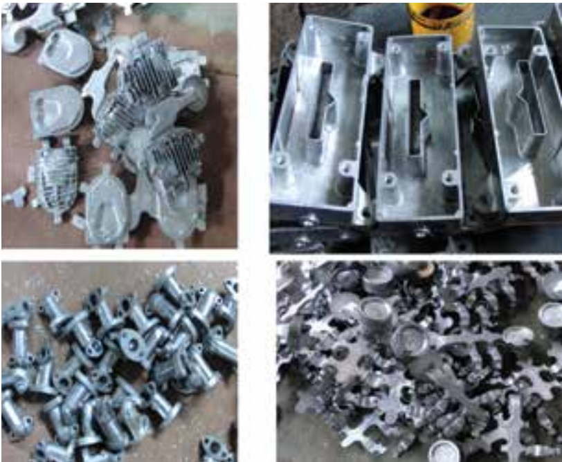
Fabricated engine parts (CYLINDER HEAD, ROCKER COVER, CARBURETTOR PARTS for Local Content Development in Automobile Industry)
